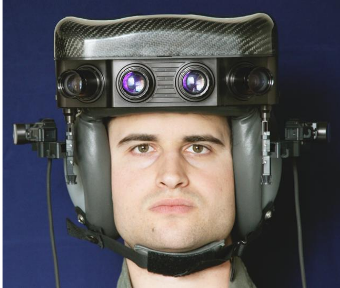
Figure 7: HRNVS with stowed eyepieces has no peripheral obscuration and a very low swept volume
