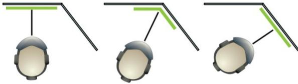
**Figure 2. Symbology Bend and Slant Provided by Manipulating Imagery Electronically on the HMD**
